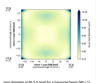
spot diameter at 86.5% level for a Gaussian beam (M² = 1) with 10.0 mm diameter at  $1/e^2$ , clipped at 10.0 mm field size and mirror distances as given above for a two mirror scan system
